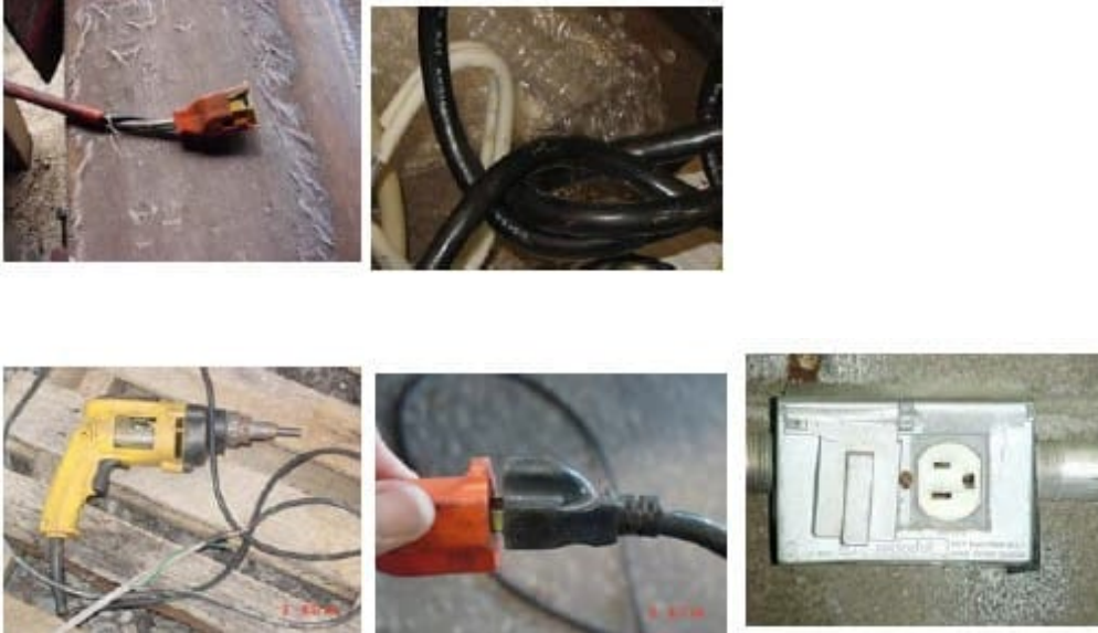
Image 4:4 Extension Cord Safety Hazard Examples. (Source: www.osha.gov , Public Domain).
