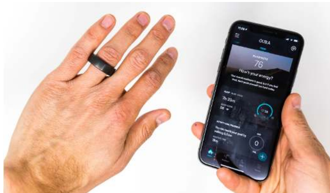
Figure 1.17: The fitness tracking ring is a new take on the fitness tracker. It can track activity and sleep cycles and send the information to your smartphone. (credit: “Left hand with Aura smart ring on finger, right hand shows phone with the Aura app’s energy and activity statistics” by Marco Verch/Flickr, CC BY 2.0)
