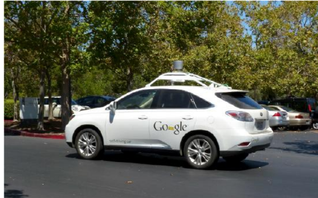
Figure 1.9: Google's Waymo, a self-driving car, can navigate roads, maintain safe speeds, and see obstacles in time to apply the brakes. (credit: "Google Self-Driving Car" by R Boed/Flickr, CC BY 2.0)
