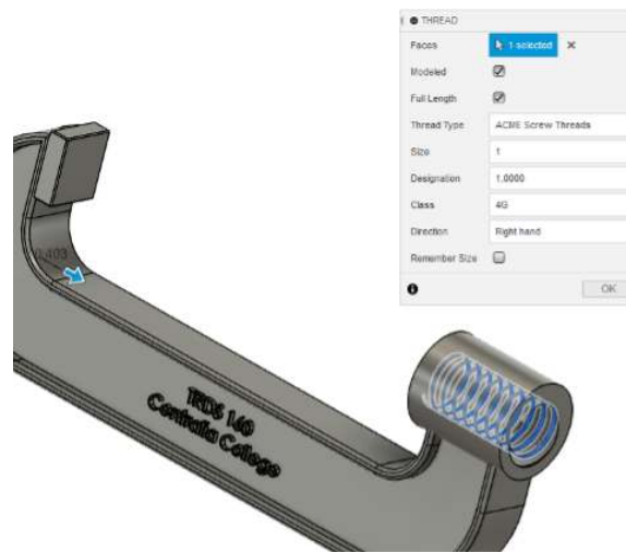
Figure 1.9.18: Add ACME threads.
