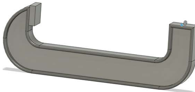
Figure 1.9.10: Fillet applied to the extruded lip.
