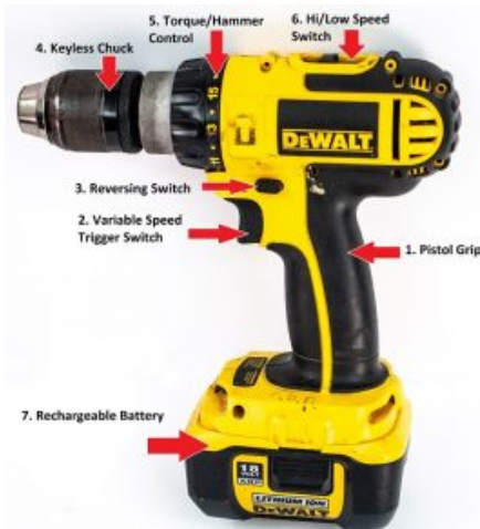
Figure 1.6.1: Portable Drill Parts by Gwen Arkin & Clifford Rutherford is licensed under CC BY 4.0
