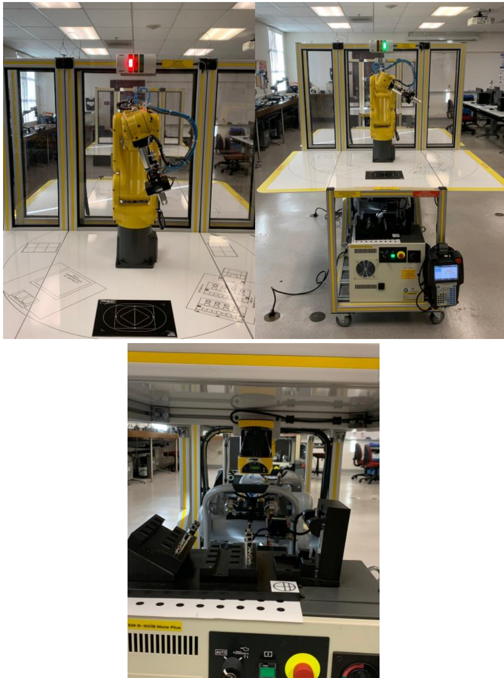
Figure 7.C.2: Robotics Lab, unsafe, safe state, safety scanner. (Source; William Oneil-Chaffey College)
