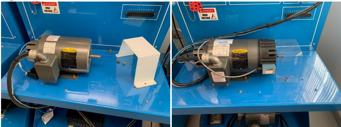
Figure 7.C.1: Motor Coupling unguarded and guarded. (Source; William Oneil-Chaffey College)
