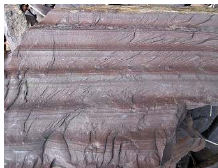
Figure 8.1.2: Varves are common sedimentary units in Pleistocene proglacial lake settings.
