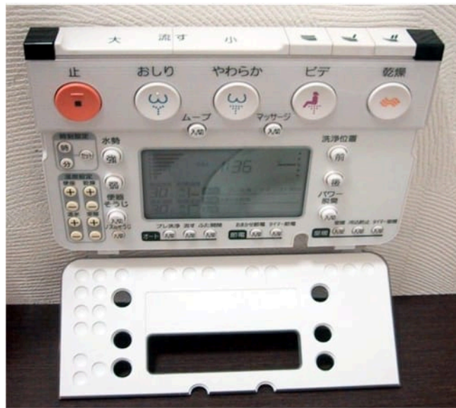
Figure 5.3.7: Wireless toilet control panel in Japan
