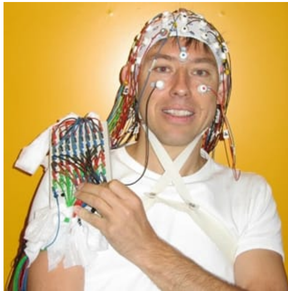
Figure 14.4.2: This man is wearing an elastic electrode cap into which individual electrodes (inside the white circles) are sewn into standardized locations. [Image: Hans, CC0 Public Domain, goo.gl/m25gce ]
