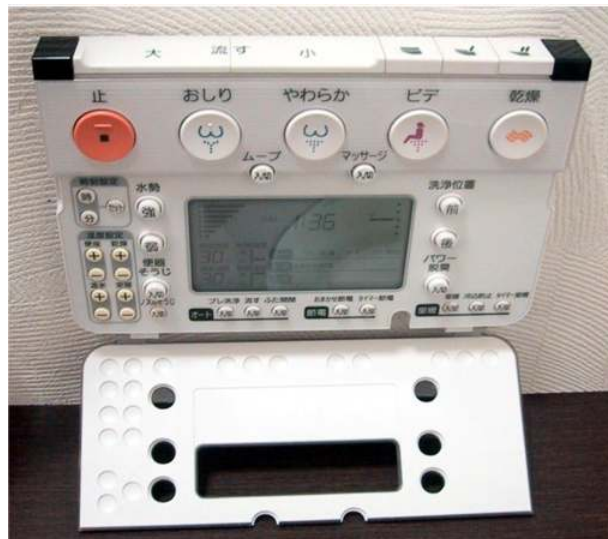
Figure 7.3.7: Wireless toilet control panel in Japan
