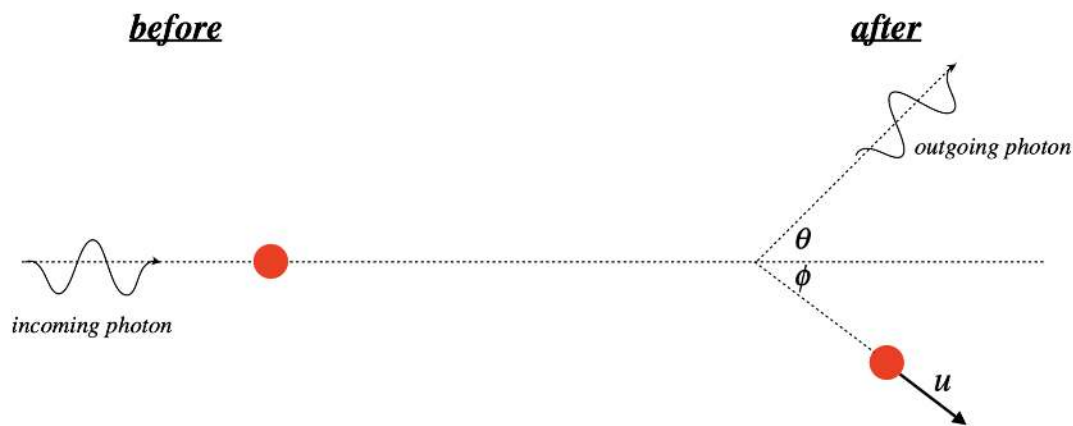
Figure 5.3.1 – Photon Scatters off a Particle
