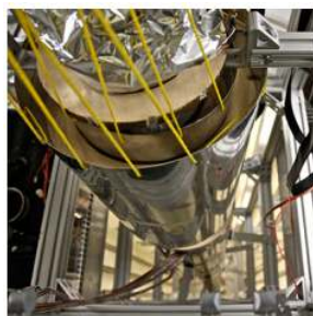
Figure 1.1.3.2: An atomic clock such as this one uses the vibrations of cesium atoms to keep time to a precision of better than a microsecond per year. The fundamental unit of time, the second, is based on such clocks. This image looks down from the top of an atomic fountain nearly 30 feet tall. (credit: Steve Jurvetson)
