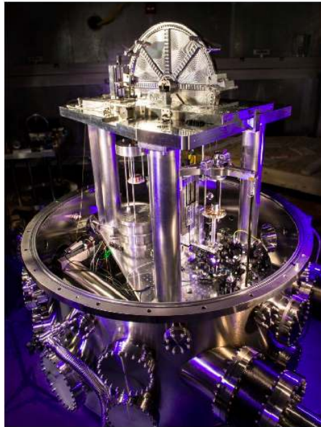
Figure 1.1.3.4: Redefining the SI unit of mass. The U.S. National Institute of Standards and Technology's Kibble balance is a machine that balances the weight of a test mass with the resulting electrical current needed for a force to balance it.
