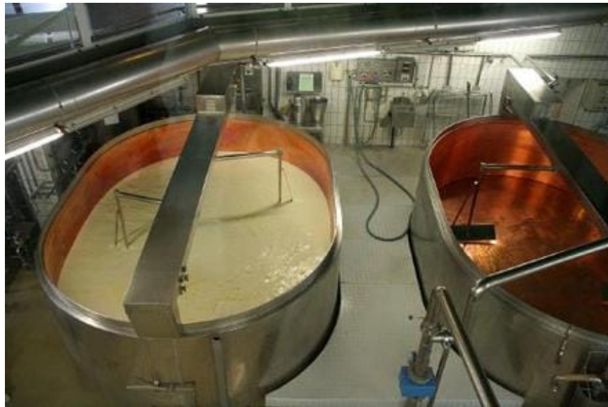
Figure 14.3.2: Industrial cheese production. 10,000 l milk in the left tank, the milk was mixed with rennet and is now broken for the production of Emmentaler.. (CC BY-SA 3.0; MatthiasKabel ).
