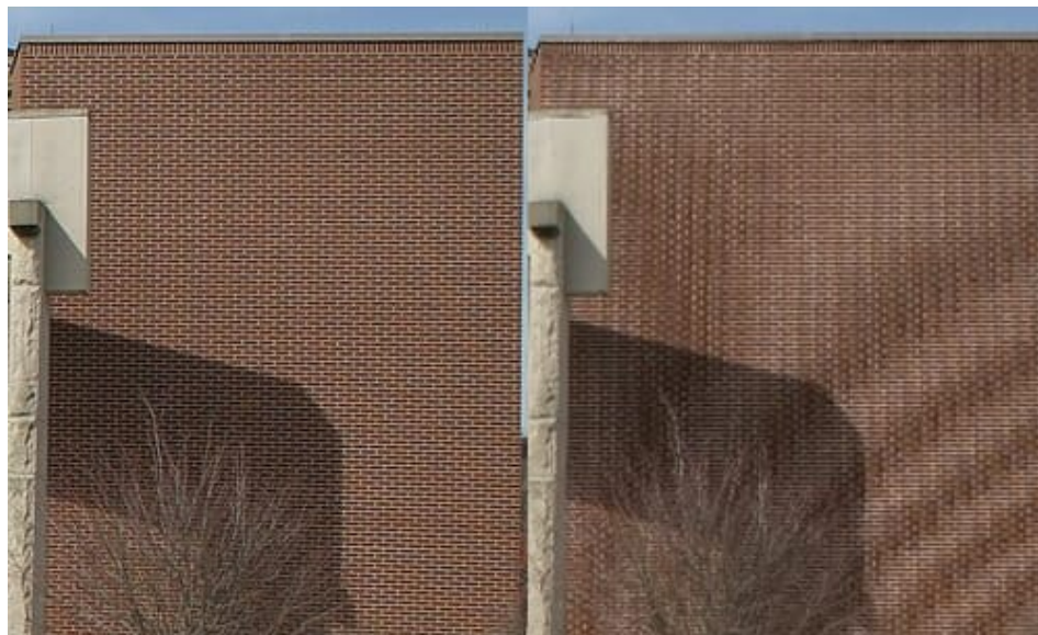
1.2.4: Original image (left) and image after jpeg compression (right) exhibiting Moiré patterns (images from Wikipedia used under CC BY-SA 3.0 license).
