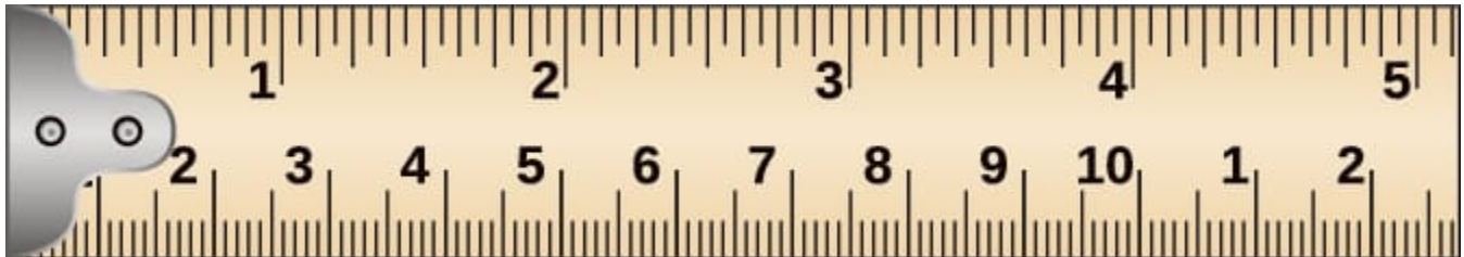
Figure 3.3.1: This tape measure measures inches along the top and centimeters along the bottom.
