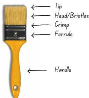
The Parts of a Paint Brush
