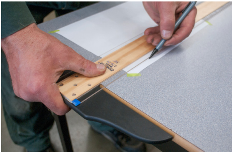
Figure 4.2.1.1.1 A person using a T-square
