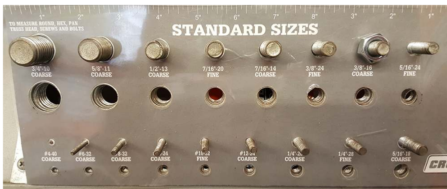
Figure 5.1.4.1 SAE Bolt Sizes by Clifford
