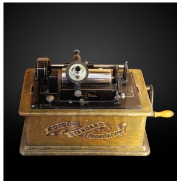
Figure 2.11 A 1901 example of Edison’s wax cylinder phonograph.
