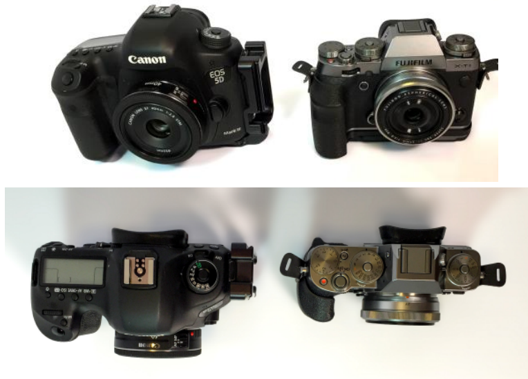
Figure 7.1.2: The DSLR (left) is taller, wider, and thicker than the Mirrorless camera (right). (CC BY-NC-ND 2.0; jbkalla via flickr)
