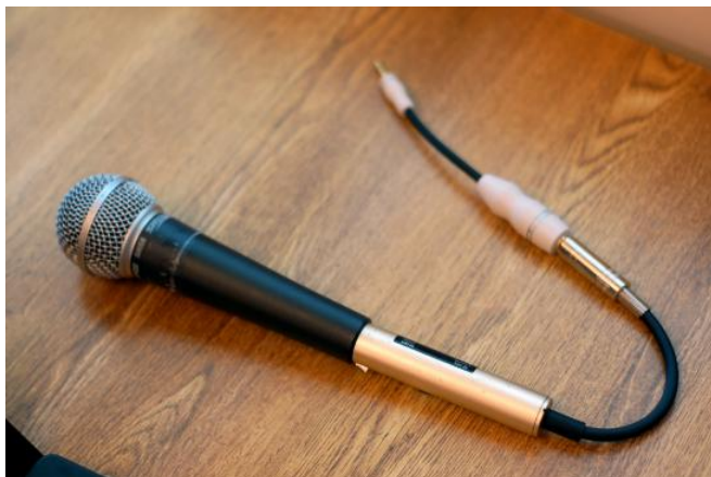
Figure 10.3.2: XLR to 1/4" Plug with 1/8" plug adapter.
