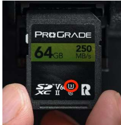
Figure 7.2.5: UHS Speed Class on an SD card. ( Unsplash License ; by Manuel Chinchilla on Unsplash )
