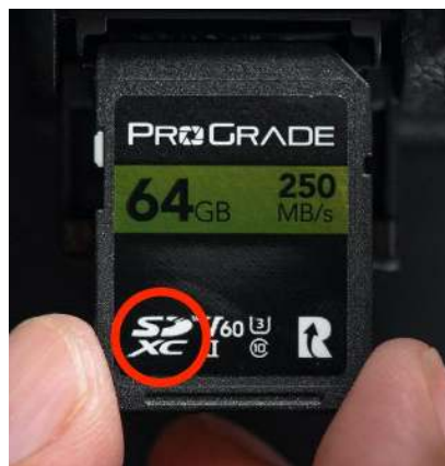
Figure 7.2.2: SD card memory format label. ( Unsplash License ; by Manuel Chinchilla on Unsplash )
