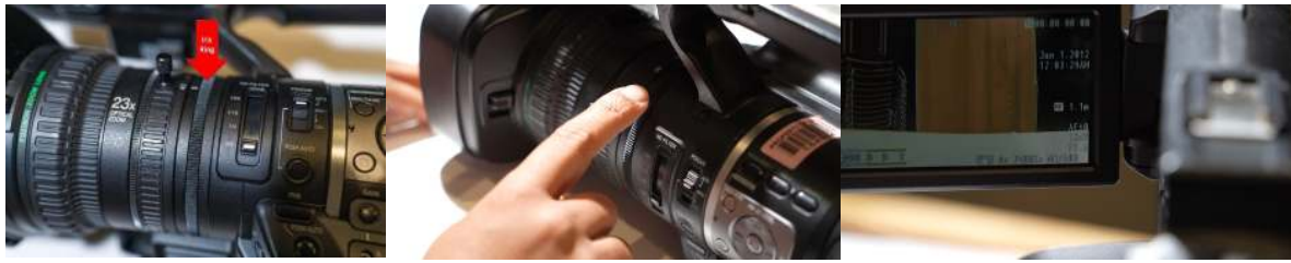
Figure 7.4.4: Iris Ring on Video Camera (left) Turning the Iris Ring (center) The effect of turning the Iris Ring on the camera image (right). (CC BY-NC 4.0; Sebastian Jimenez via San Francisco State University)
