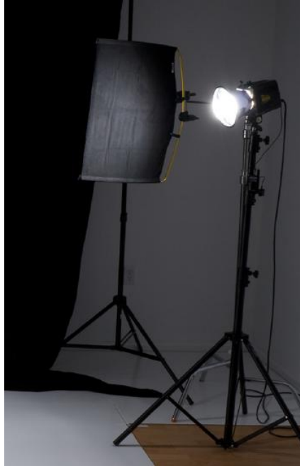
Figure 9.5.5: Flag blocking light from hitting the backdrop. (CC BY 2.0; Tim Johnson via Wikimedia Commons)
