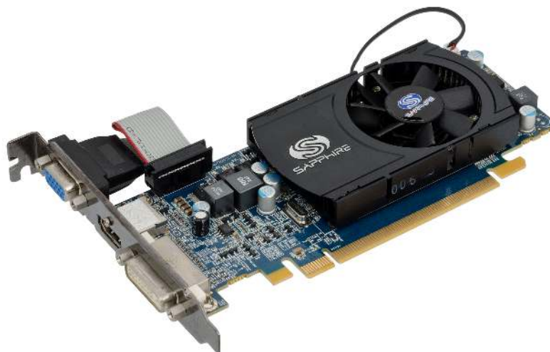
Figure 11.1.2: Sapphire-brand, Radeon HD 5570 video graphics card, for computer graphics. (Copyright; Public Domain
