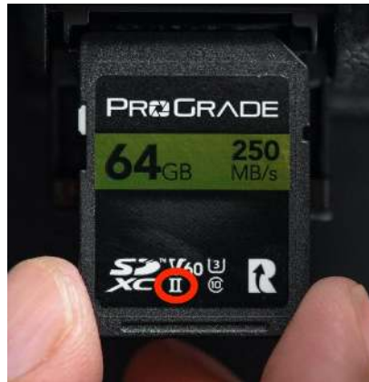
Figure 7.2.3: UHS rating on an SD card. ( Unsplash License ; by Manuel Chinchilla on Unsplash )
