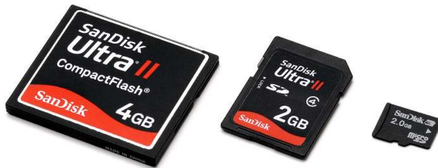
Figure 7.2.1: Size comparison of CF, SD, and MicroSD cards. (Public Domain; Evan-Amos via Wikimedia Commons )
