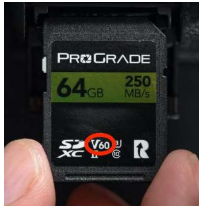
Figure 7.2.6: Video Speed Class on an SD card. ( Unsplash License ; by Manuel Chinchilla on Unsplash )
