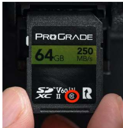
Figure 7.2.4: Speed Class rating on an SD card. ( Unsplash License ; by Manuel Chinchilla on Unsplash )
