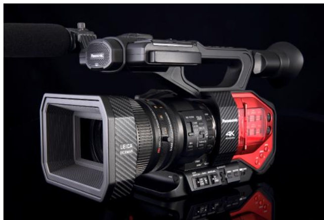
Figure 7.1.3: Video Camcorders are longer than DSLR and Mirrorless cameras with many of the needed functions placed on the side. (Public Domain Mark 1.0; Teixeira, Paulo via flickr)
