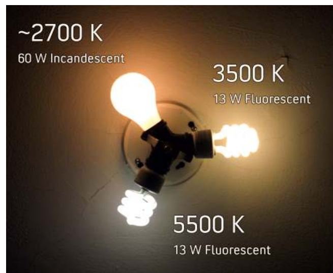
Figure 7.10.3: At 2700K the light in the top left has an orange tint; At 3500 the second light on the right has a yellow tint; at 5500K the light on the bottom left has a blue tint. (Public Domain; Yurocuc via Wikimedia)
