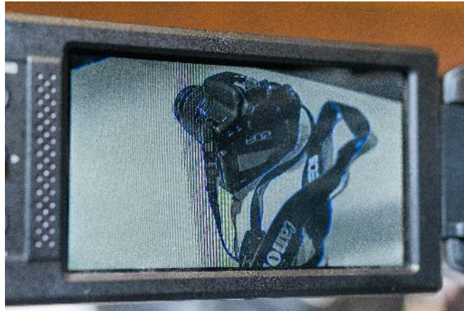
Figure 7.8.3: When the Focus Assist is in use, the image turns black and white, and blue lines appear around objects in focus. (CC BY-NC 4.0; Sebastian Jimenez via San Francisco State University)
