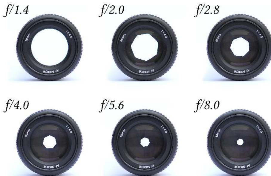
Figure 7.4.1: Apertures get smaller as the and f-stops increase (CC BY-SA 4.0 International; KoeppiK via Wikimedia)
