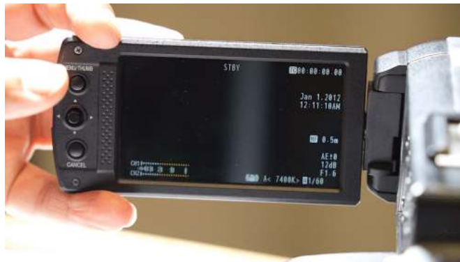
Figure 7.2.1.2: Using the internal menu in a video camera to format an SD card. ( CC BY-NC 4.0 ; Sebastian Jimenez via San Francisco State University)
