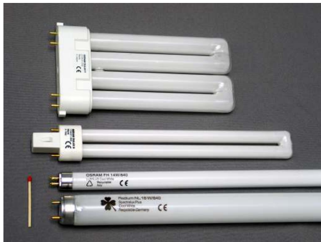
Figure 9.2.2: Florescent light bulbs in two shapes and thicknesses. (CC BY-SA 2.0 DE; Christian Taube via Wikimedia Commons )
