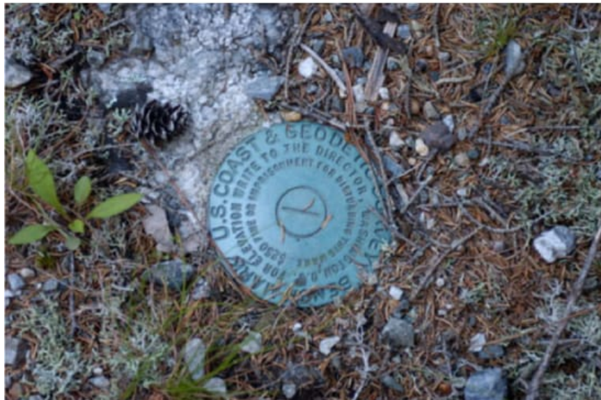
Figure 4.6: A survey marker at the peak of Isle of Springs, Maine. Geodetic markers such as this are geographic reference points marked by 3 1/2 inch disks in ground-level concrete cylinders. These markers are located at precise coordinates throughout the world.
