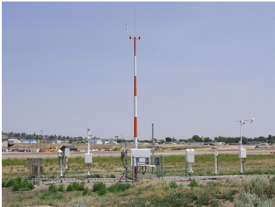
Electrical thermometers are used in systems such as this Elko Automated Surface Observing System (ASOS) ( CC BY-SA 3.0 ).
