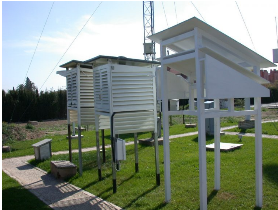
These meteorological shelters protect the instruments inside while still allowing a fairly accurate collection of data ( CC BY 3.0 ).
