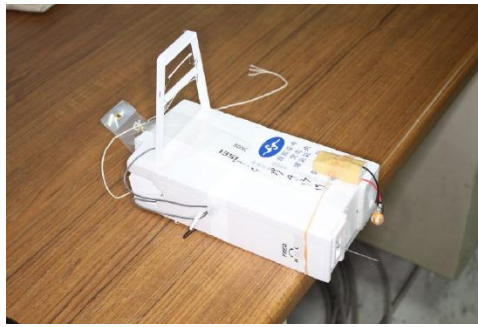
Radiosondes contain thermistor temperature sensors ( CC BY-SA 3.0 ).
