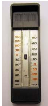
Minimum and maximum mercury thermometer ( CC BY-SA 3.0 ).
