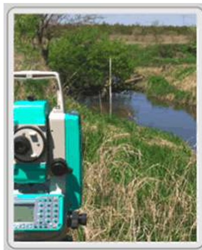
Figure 2.11: Total station, a surveying instrument, measures distance, direction, and location. Image comes from Illinois State University, Geography Dept.
