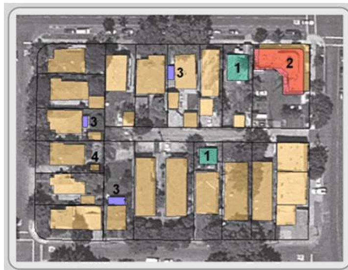
Figure 3.16: Map verification: 1 = layer is missing building. 2 = building's position needs to be altered. 3 = layer may be missing buildings (check with additional sources or field check). 4 = layer depicts building that does not exist.
