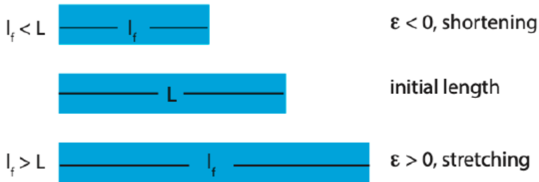
Figure 1.2.2: Normal strain leads to shortening or stretching of an object.
