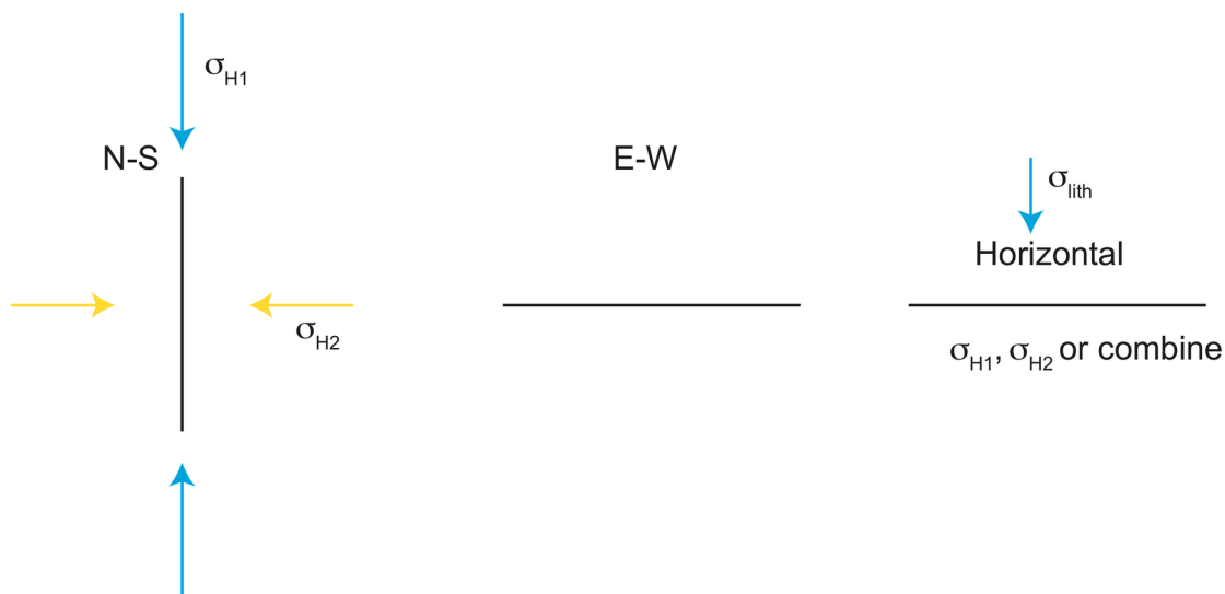
Figure 1.4.5: Example of plane orientations with no shear stress. The normal stresses acting across these planes are principal stresses.
