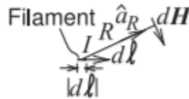
Figure 1.1.3: Diagram illustrating the Biot-Savart law. The law relates a static filament of current to the incremental H field at a distance.
