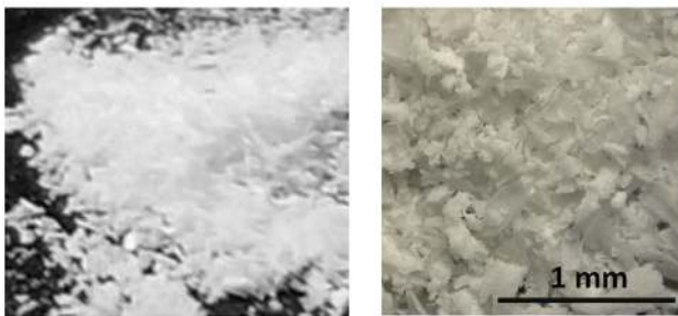
At 20 mm Drilling Depth: Powdery Chip Type
