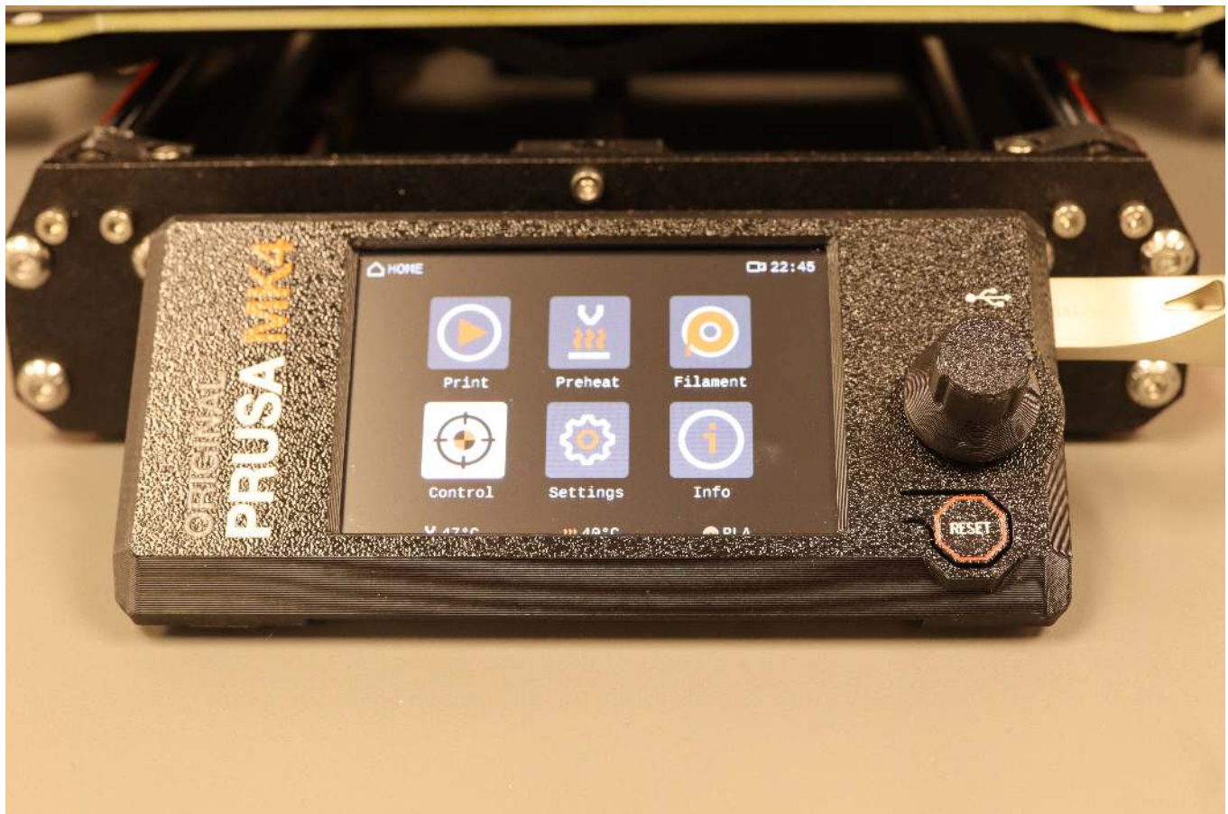
Figure 4.3.2: Prusa Mk. 4 Console displaying the Print, Preheat, Filament, Control, Settings and Info menu options.
