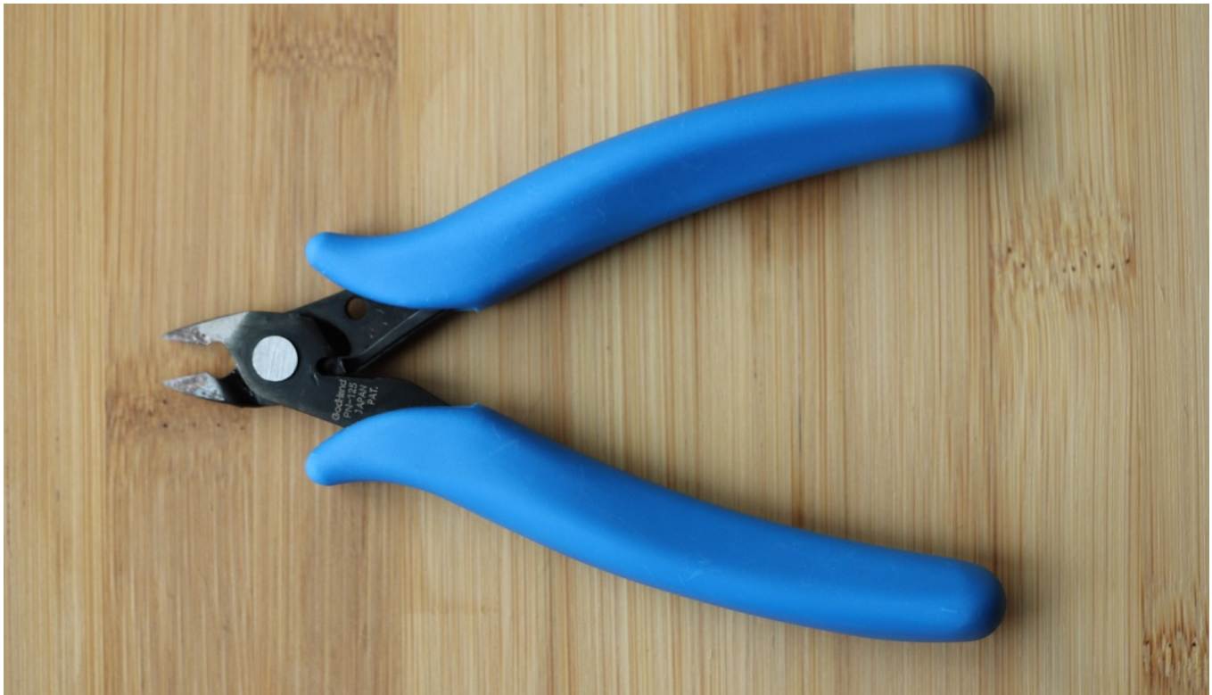
Figure 4.6.1: A pair of wire cutters commonly used to clean up 3D Prints
