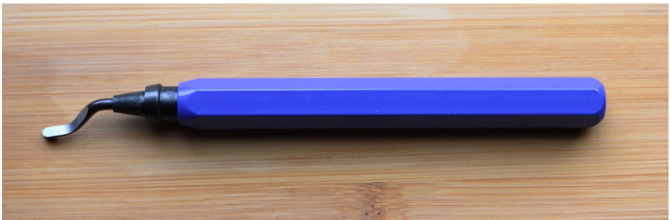
Figure 4.6.1: Deburring tool used to clean up the edges of 3D prints
