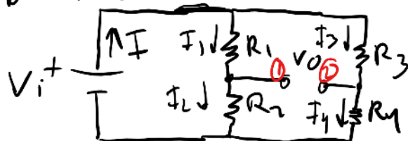
Figure Chapter6.5: Voltage at Position 1 and 2 in Wheatstone Bridge and Voltage Dividing Circuits.
