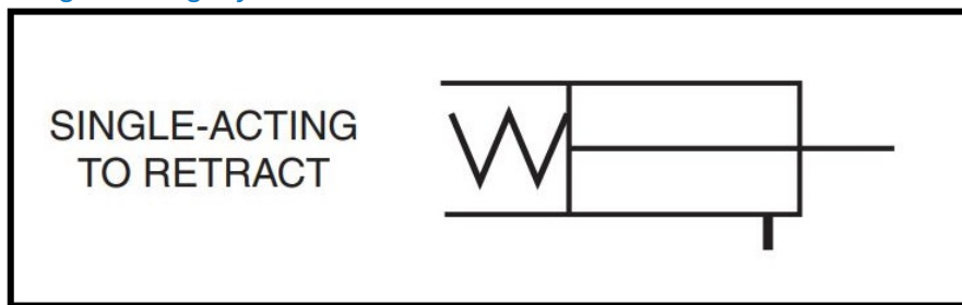
Figure 6.2.2: A pneumatic schematic of a spring-extension single-acting cylinder (ISO 1219).
