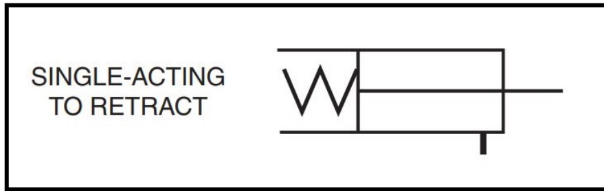
Figure 6.3.1: A pneumatic schematic of a spring-extension single-acting cylinder (ISO 1219).
