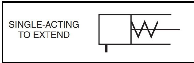
Figure 6.2.1: A pneumatic schematic of a spring-return single-acting cylinder (ISO 1219).
