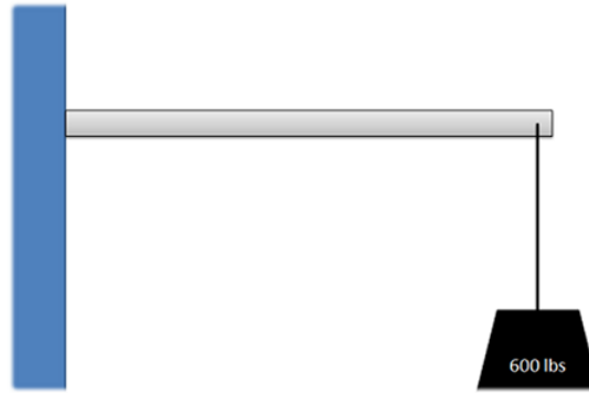
Figure 1.6.10: problem diagram for Example 1.6.4; a 600-lb load hangs from the free end of a horizontal beam whose other end is attached to a wall.
