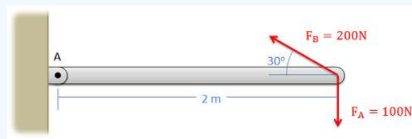
Figure 3.1.6: problem diagram for Example 3.1.1; a lever is attached to a wall with two forces exerted upon the lever's free end.
