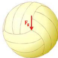
Figure 2.2.3: Though gravitational forces are technically body forces, they are often approximated as a single point force acting on the center of gravity of the object. Adapted from Public Domain image, no author listed.
