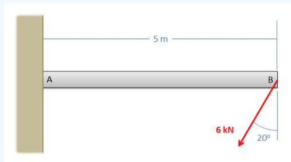
Figure 3.4.2: problem diagram for Example 3.4.2. A horizontal beam attached to the wall at one end experiences a force applied at its free end.
