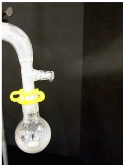
Figure 5.33: Vapor escaping from vacuum adapter.
