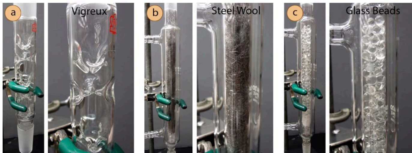
Figure 5.39: Different fractionating columns: a) Vigreux, b) Steel wool, c) Glass beads.
