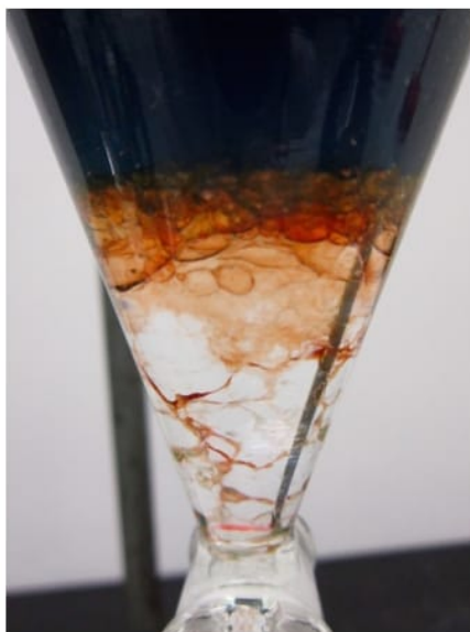
Figure 4.33: Emulsion formed between dichloromethane and brine (with food coloring).
