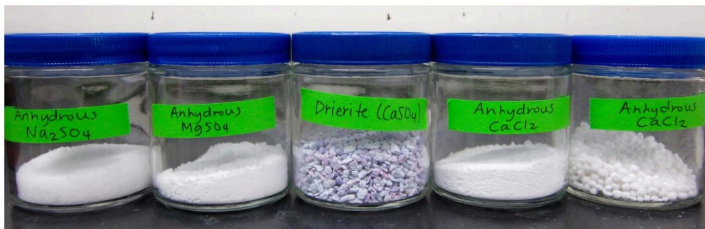
Figure 4.48: Various drying agents: Anhydrous Na_2SO_4 , anhydrous MgSO_4 , Drierite CaSO_4 , and anhydrous CaCl_2 .
