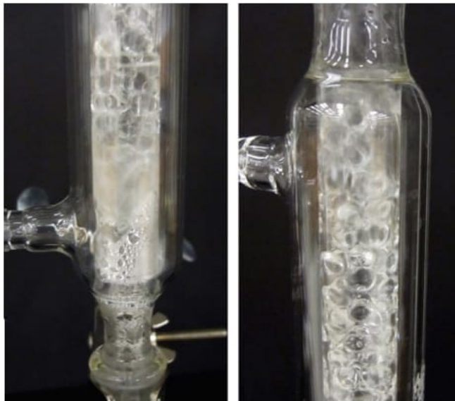
Figure 5.45: Flooding of a fractionating column.
