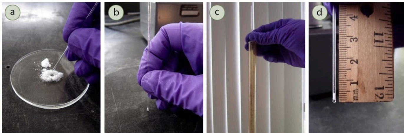
Figure 6.10: a) Depositing sample into the open end of a capillary tube, b) Inverting and tapping the tube on the benchtop, c) Dropping the sample through a long tube, d) Correct height of sample in the tube.
