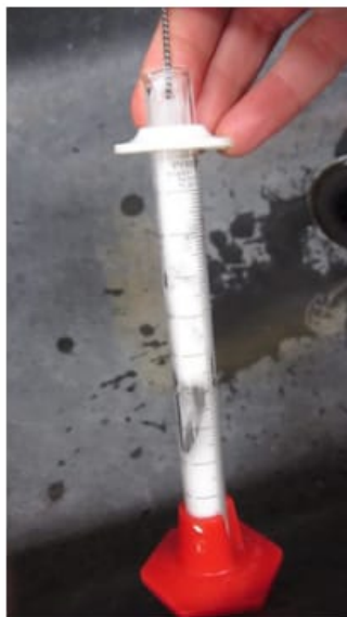
Figure 1.10: Detergent foaming during washing.
