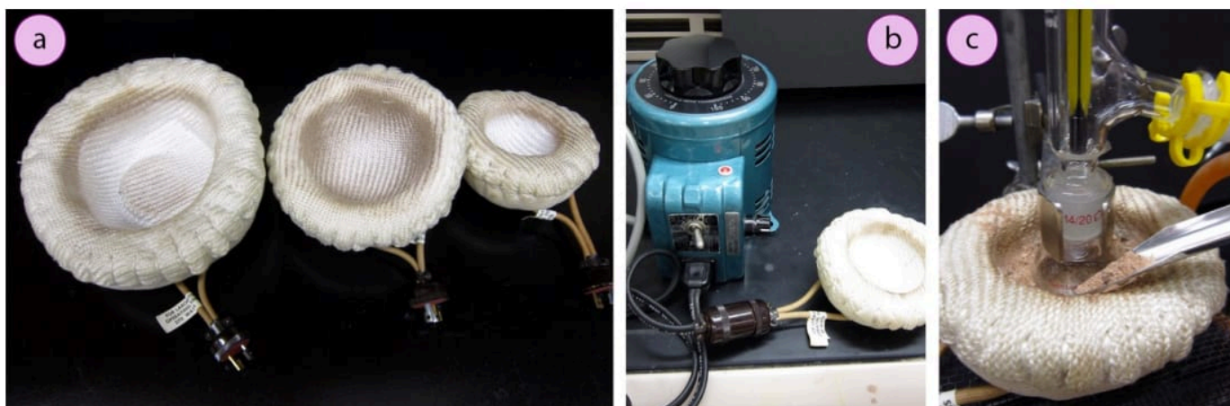
Figure 1.51: a) Three sizes of heating mantle, b) Heating mantle connected to a Variac, c) Filling a heating mantle with sand.
