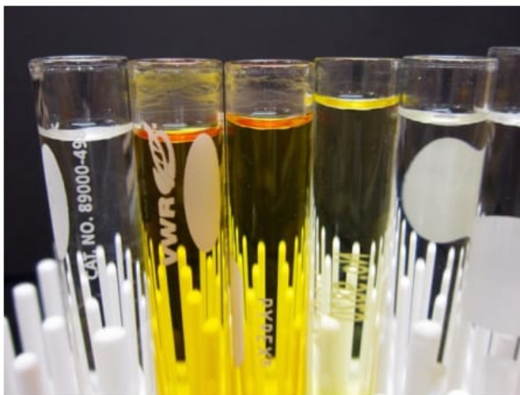
Figure 2.62: Ring of solid seen on tube rims after evaporation.
