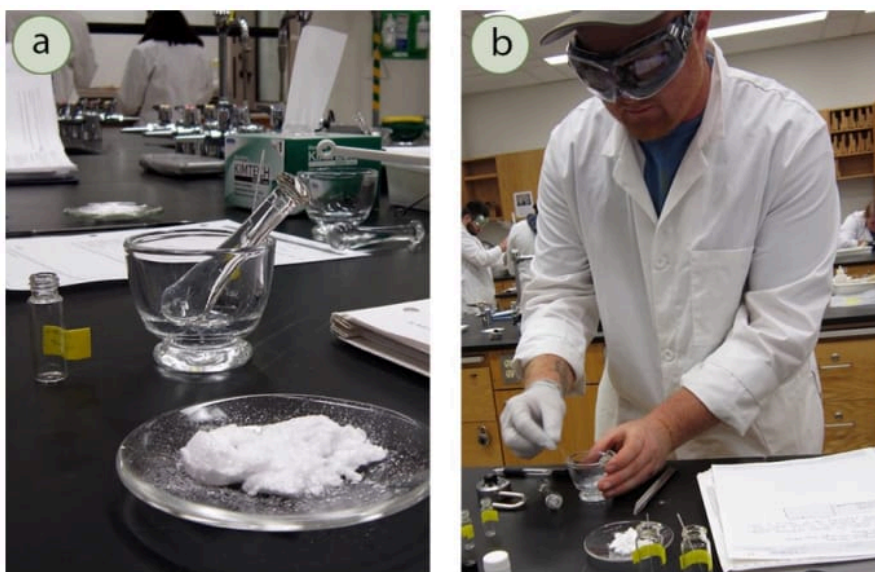
Figure 6.18: a) Mortar and pestle in front of sample, b) A student prepares a sample for a mixed melting point.
