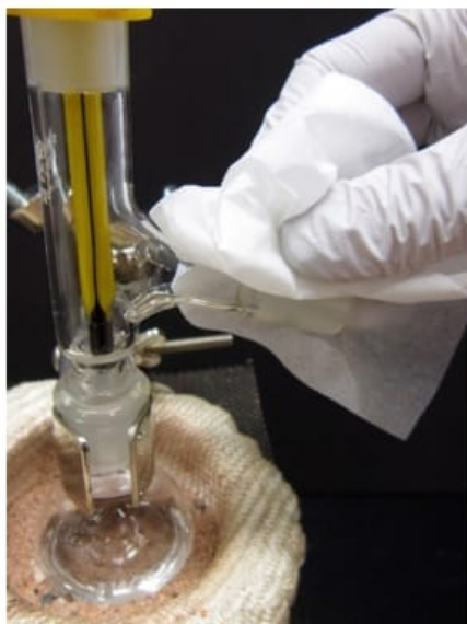
Figure 1.9: Removing grease with a KimWipe soaked in hexanes.
