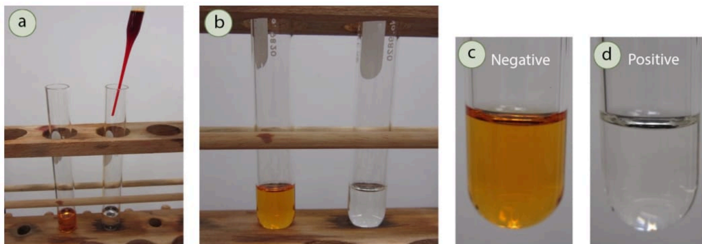
Figure 6.54: a) Addition of the bromine solution (orange liquid) to a test tube, b) Bromine results: hexanes (left tube), 1-hexene (right tube), c) Negative result, d) Positive result.
