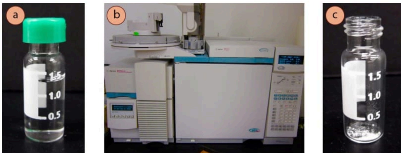
Figure 2.93: a) GC vial, b) GC-MS instrument, c) Small amount of solid in a GC vial.
