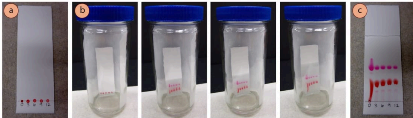
Figure 2.22: a) Red food dye spotted at different dilutions, b) Elution, c) Developed TLC plate.
