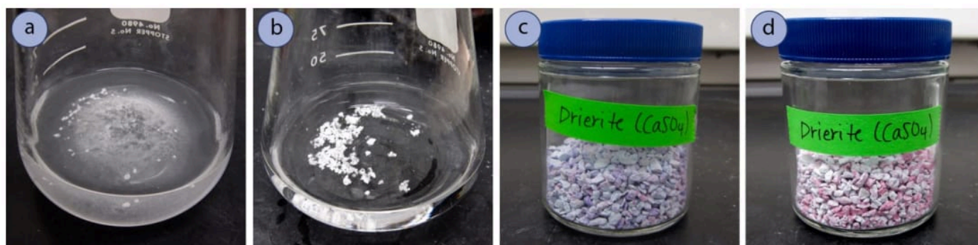
Figure 4.49: a) Ethyl acetate solution containing fine particles of anhydrous MgSO_4 , b) Ethyl acetate with clumpy MgSO_4 hydrate, c) Dry Drierite (blue), d) Wet Drierite (pink).
