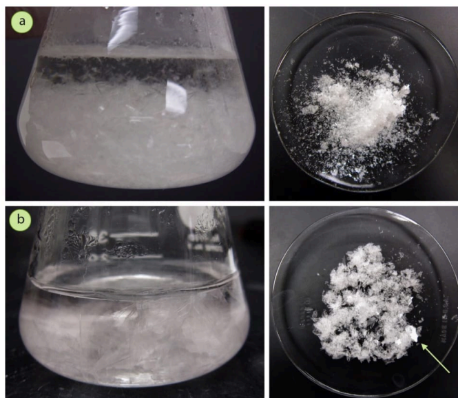
Figure 3.17: a) These crystals of acetanilide formed from water are perfectly acceptable, but small, b) These crystals of acetanilide were grown much more slowly, and are larger (note crystal indicated with the arrow).
