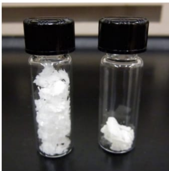
Figure 3.37: First crop crystals of 4-bromoacetophenone (left) and second crop crystals (right).
