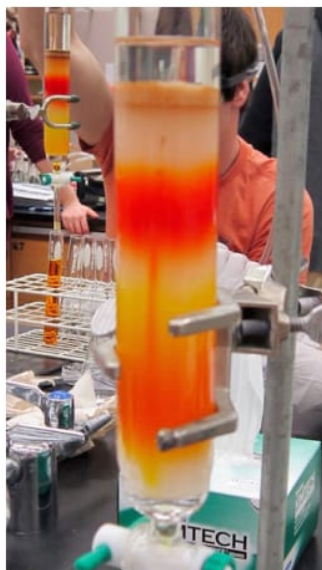
Figure 2.65: Effect of a broken pipette on a column.
