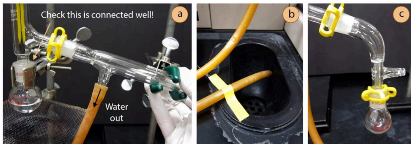
Figure 5.24: a) Connection of the condenser to the three-way adapter (with arrow pointing to the joint that needs to be very secure for safety reasons), b) Securing water hoses to the sink with lab tape, c) Attachment of the vacuum adapter and receiving flask.
