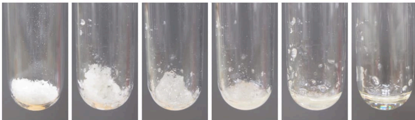
Figure 6.6: Time-lapse melting of a mixture of piperonal and resorcinol at room temperature (both are white solids when pure). Note: no heat is applied in the process. The mixture eventually melts as a result of its depressed melting point.
