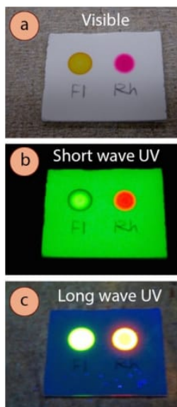
Figure 2.32: Fluorescein and rhodamine B solutions viewed with: a) Visible light, b) Short-wave UV, c) Long-wave UV.
