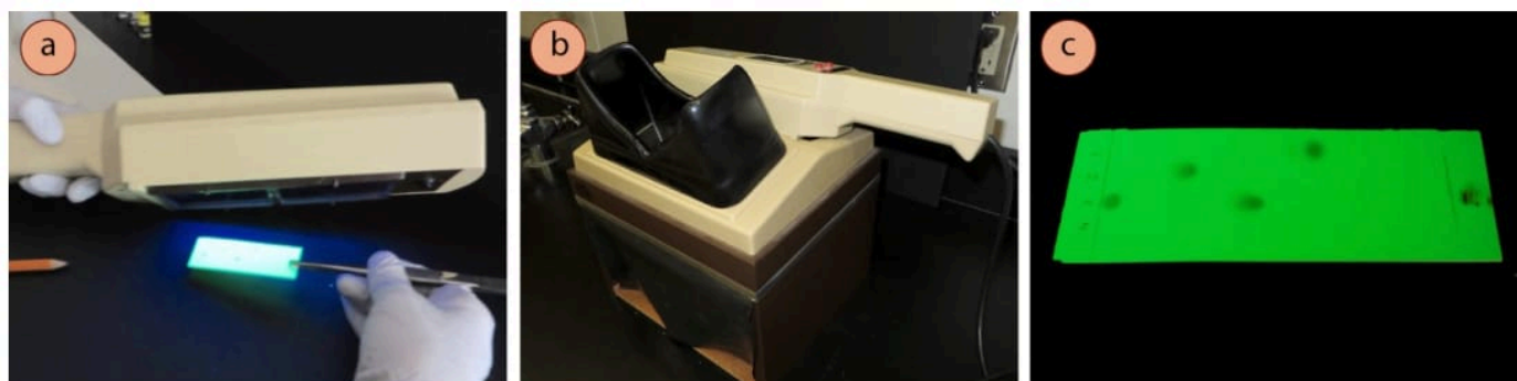
Figure 2.31: a) Tilting a UV lamp to visualize a TLC plate, b) Box to protect eyes from UV damage, c) Appearance under UV.
