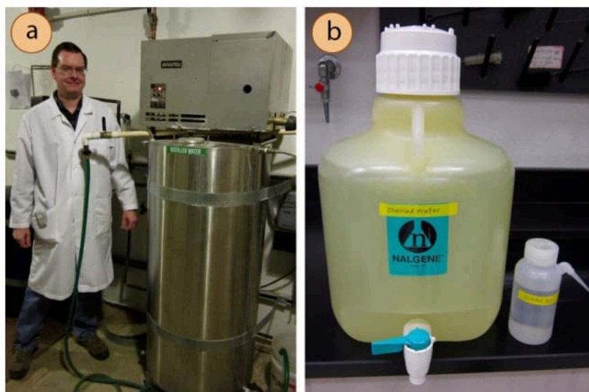
Figure 5.5: a) Distilled water generator at Butte College. The top metallic box is the actual generator, and the bottom cylindrical container is the reservoir, b) Distilled water carboy and wash bottle.
