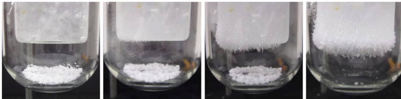
Figure 7.14: Vacuum sublimation sequence.
