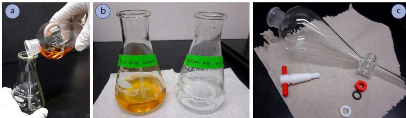
Figure 4.28: a) Pouring out the top layer, b) Labeled layers, c) Drying the separatory funnel with a disassembled stopcock.
