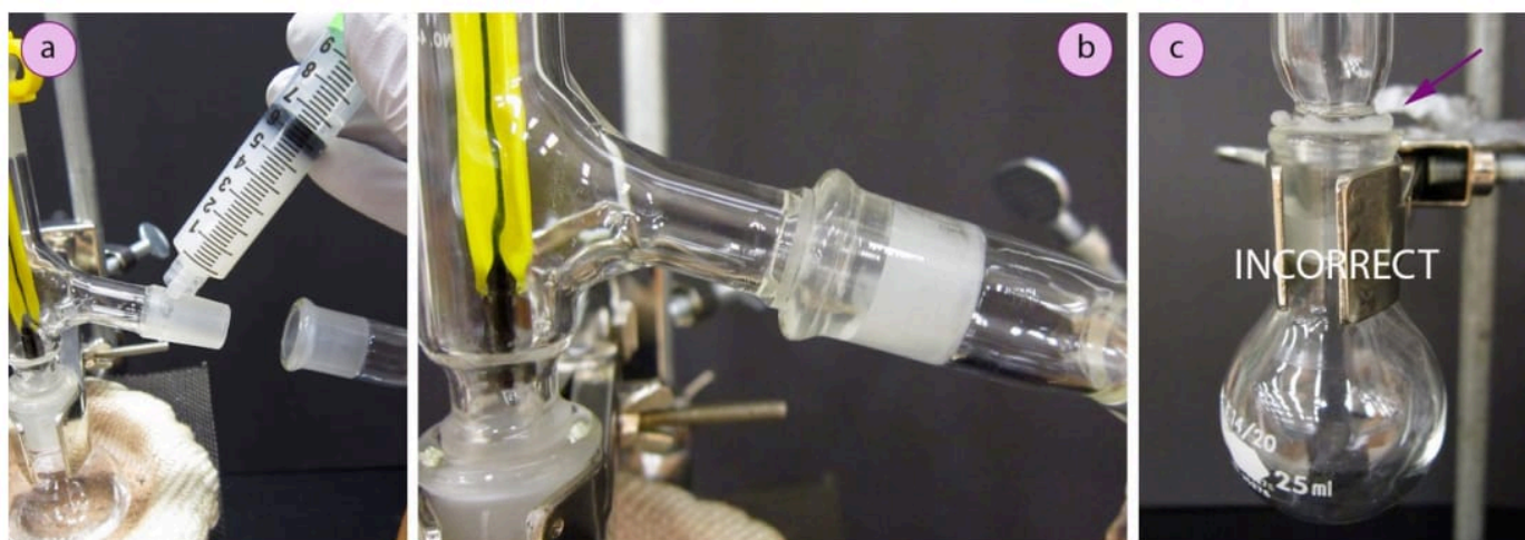
Figure 1.8: a) Applying grease by syringe, b) Properly greased joint, c) Too much grease in the joint, as indicated with an arrow.
