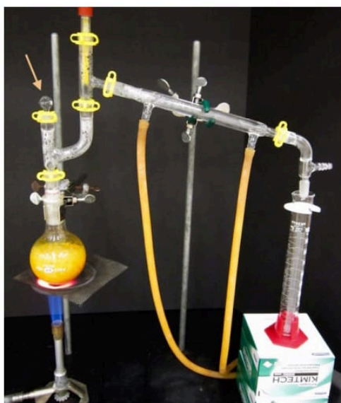
Figure 5.60: Steam distillation variation where sufficient water will be used. The arrow indicates a stopper used to close the system.
