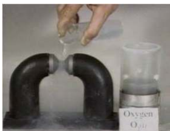
Figure 11.5. Demonstration showing blue liquid O_2 attracted to the poles of a permanent magnet. From jchemed.chem.wisc.edu/jcsoft.../PARANIO/9.HTM
