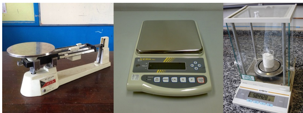
Figure 2.1.2 (From left to right:) Triple beam balance ( source(opens in new window) ), digital top-loading balance ( source(opens in new window) ), and an analytical balance ( source ).
