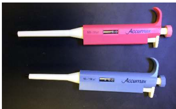
Figure 1.1.5 : A set of two digital micropipettes. The pipet on the top delivers volumes between 0.5 mL and 10 \mu L and the pipet on the bottom delivers volumes between 10 mL and 100 \mu L.
