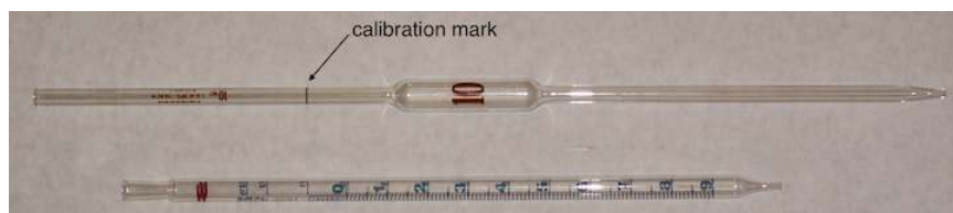
Figure 1.1.4 : Two examples of 10-mL volumetric pipets. The pipet on the top is a transfer pipet and the pipet on the bottom is a Mohr measuring pipet. The transfer pipet delivers a single volume of 10.00 mL when filled to its calibration mark. The Mohr pipet has a mark every 0.1 mL, allowing for the delivery of variable volumes. It also has additional graduations at 11 mL, 12 mL, and 12.5 mL.
