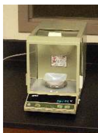
Figure 1.1.1 : The photo shows a typical digital electronic balance capable of determining mass to the nearest \pm 0.1 mg. The sticker inside the balance's wind shield is its annual calibration certification. For a review of other types of electronic balances, see Schoonover, R. M. Anal. Chem. 1982 , 54, 973A-980A.
