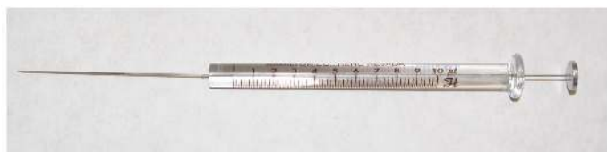
Figure 4.1.8 . Example of a syringe for injecting samples into a gas chromatograph. This syringe has a maximum capacity of 10 \mu\text{L} with graduations every 0.1 \mu\text{L} .
