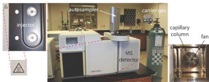
Figure 4.1.1 . Example of a typical gas chromatograph with insets showing the heated injection ports—note the symbol indicating that it is hot—and the oven that houses the column. This particular instrument is equipped with an autosampler for injecting samples, a capillary column, and a mass spectrometer (MS) as the detector. Note that the carrier gas is supplied by a tank of compressed gas.
