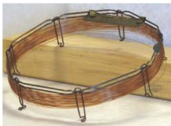
Figure 4.1.3 . Typical example of a capillary column for gas chromatography. This column is 30 m long with an internal diameter of 247 \mu\text{m} . The interior surface of the capillary has a 0.25 \mu\text{m} coating of the liquid phase.
