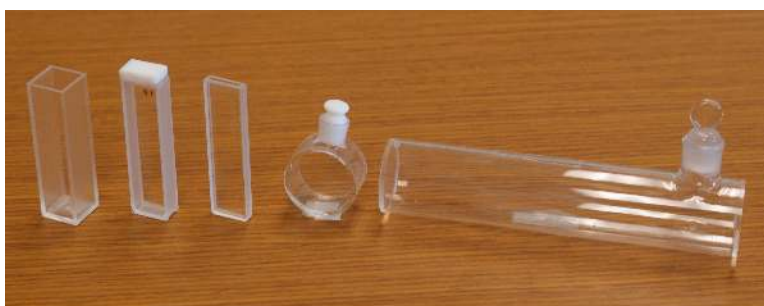
Figure 2.2.6. Examples of sample cells for UV/Vis spectroscopy. From left to right (with path lengths in parentheses): rectangular plastic cuvette (10.0 mm), rectangular quartz cuvette (5.000 mm), rectangular quartz cuvette (1.000 mm), cylindrical quartz cuvette (10.00 mm), cylindrical glass cuvette with quartz windows (100.0 mm). Cells often are available as a matched pair, which is important when using a double-beam instrument.
