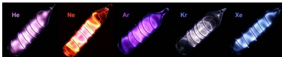
Figure 2.2.6: Glowing noble gases in glass vials with low pressure inside. Power supply: 5 kV, 20 mA, 25 kHz. Source: New work Alchemist-hp (talk) www.pse-mendelejew.de ; original single images: Jurii, http://images-of-elements.com . / CC BY ( https://creativecommons.org/licenses/by/3.0 )
