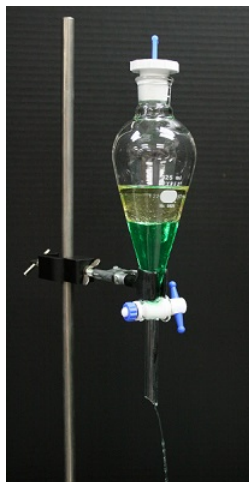
Figure 1.7.1: Separatory Funnel containing oil and colored water to display density differences. (CC BY-SA 3.0; PRHaney via Wikipedia).
