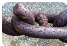
Figure 3.1.2.3: Rust (iron oxide) forms on an unprotected iron surface.
