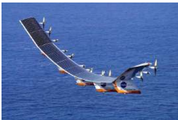
Figure 4.3.3.1.2: Solar energy is converted into electrical energy by solar cells, which is used to run a motor in this solar-power aircraft. (credit: NASA)
