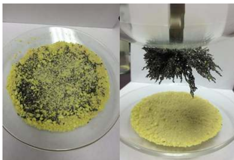
Figure 2.1.4: A heterogeneous mixture of iron and sulfur (left), separated by a magnet (right). Source: Asoult / CC BY ( https://creativecommons.org/licenses/by/4.0 )
