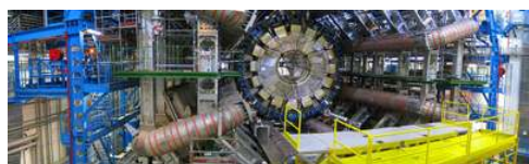
Figure 4.2.5.3: The world's largest particle accelerator spans the border between Switzerland and France. Two beams, traveling in opposite directions close to the speed of light, collide in a tube similar to the
