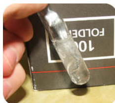
Figure 3.1.2.5: Zinc reacts with hydrochloric acid to produce bubbles of hydrogen gas.
