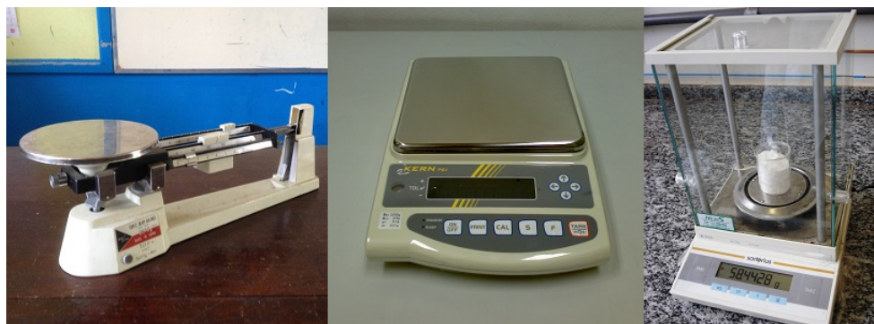
Figure 1.5.2: Triple beam balance (image from: upload.wikimedia.org/wikipedia/m_balance2.JPG . Digital top-loading balance ( upload.wikimedia.org/wikipedia/00-2M_-_01.jpg ) and an analytical balance ( upload.wikimedia.org/wikipedia/NaCl-1mol.jpg )
