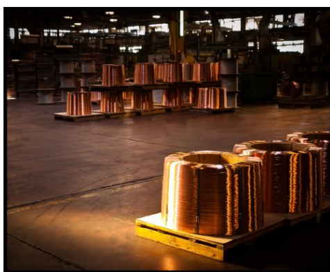
Figure 3.2.3: Metallic bonds explain many of the properties of metals. This coil of wire is made of the metal copper. Like other metals, copper is shiny, can be formed into wires, and conducts electricity. (CC BY 2.0; Flavio~ - "Industrial Photography: Copper Wires-003" via Flickr)
