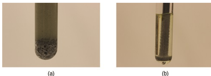
Figure 3.2.1: (a) Iron powder reacts rapidly with dilute hydrochloric acid and produces bubbles of hydrogen gas because the powder has a large total area: 2\text{Fe(s)} + 6\text{HCl(aq)} \rightarrow 2\text{FeCl}_3\text{(aq)} + 3\text{H}_2\text{(g)} . (surface) An iron nail reacts more slowly.
