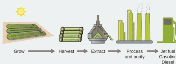
Figure 2.3.5: Algae convert sunlight and carbon dioxide into oil that is harvested, extracted, purified, and transformed into a variety of renewable fuels.
