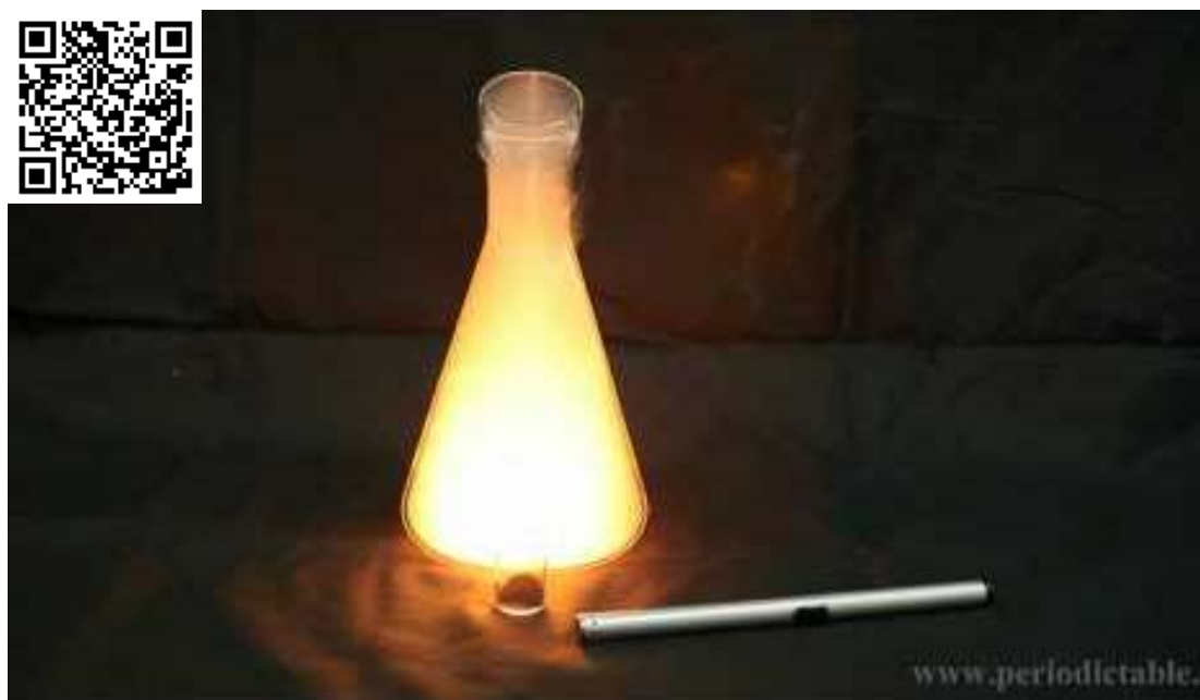
Video 3.2.2: Phosphorous burns rapidly in air, but it will burn even more rapidly if the concentration of oxygen in is higher.
