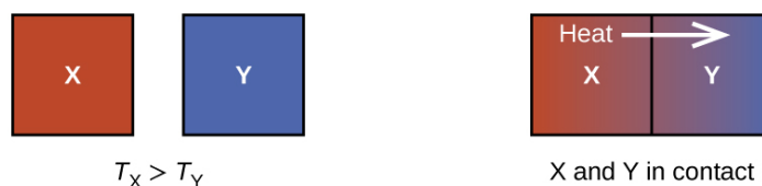
Figure 2.5.4: When two objects at different temperatures come in contact, heat spontaneously flows from the hotter to the colder object.
