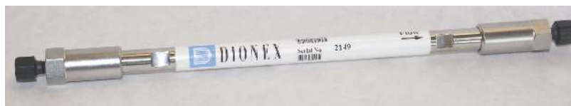
Figure 12.5.2 . Typical packed column for HPLC. This particular column has an internal diameter of 4.6 mm and a length of 150 mm, and is packed with 5 \mu\text{m} particles coated with stationary phase.
