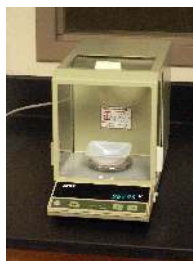
Figure 2.4.1 : The photo shows a typical digital electronic balance capable of determining mass to the nearest \pm 0.1 mg. The sticker inside the balance's wind shield is its annual calibration certification. For a review of other types of electronic balances, see Schoonover, R. M. Anal. Chem. 1982 , 54, 973A-980A.
