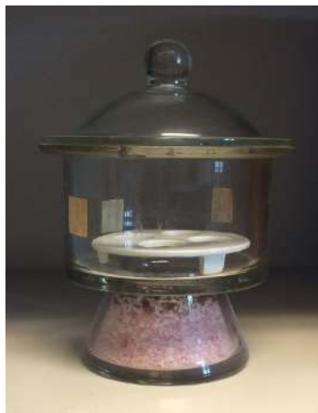
Figure 2.4.9 : Example of a desiccator. The solid in the bottom of the desiccator is the desiccant, which in this case is silica gel.
