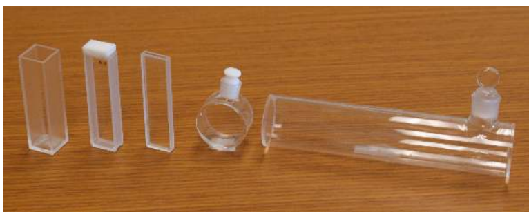
Figure 10.3.6 . Examples of sample cells for UV/Vis spectroscopy. From left to right (with path lengths in parentheses): rectangular plastic cuvette (10.0 mm), rectangular quartz cuvette (5.000 mm), rectangular quartz cuvette (1.000 mm), cylindrical quartz cuvette (10.00 mm), cylindrical glass cuvette with quartz windows (100.0 mm). Cells often are available as a matched pair, which is important when using a double-beam instrument.
