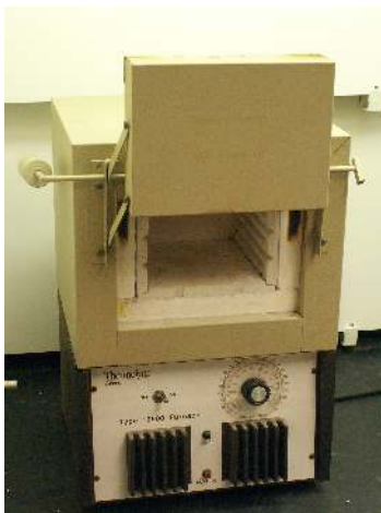
Figure 2.4.8 : Example of a muffle furnace.
