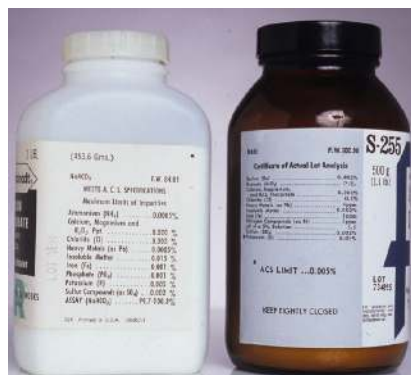
Figure 5.1.1 : Two examples of packaging labels for reagent grade chemicals. The label on the bottle on the right provides the manufacturer's assay for the reagent, NaBr. Note that potassium is flagged with an asterisk (*) because its assay exceeds the limit established by the American Chemical Society (ACS). The label for the bottle on the left does not provide an assay for impurities; however it indicates that the reagent meets ACS specifications by providing the maximum limits for impurities. An assay for the reagent, NaHCO 3 , is provided.
