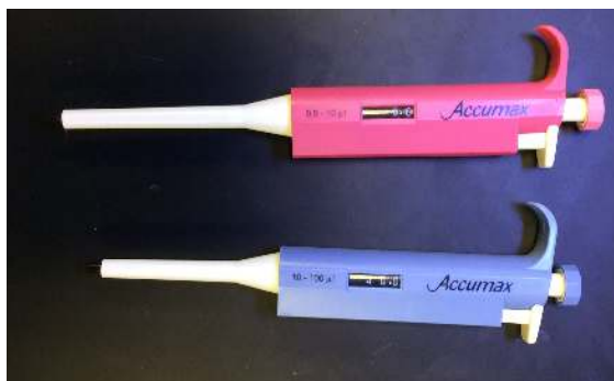
Figure 2.4.4 : A set of two digital micropipets. The pipet on the top delivers volumes between 0.5 mL and 10 \mu L and the pipet on the bottom delivers volumes between 10 mL and 100 \mu L.
