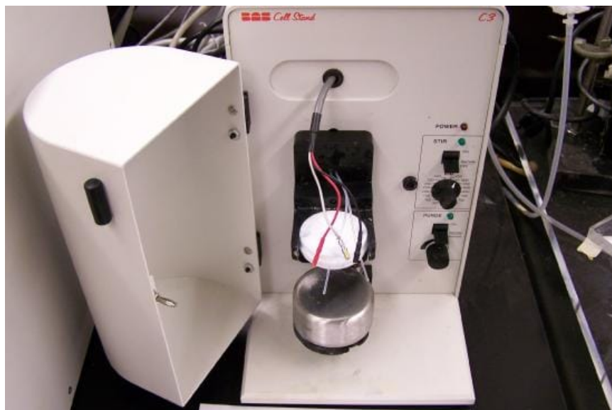
Figure 1.7: UCD cyclic voltammetry Instrument (including potentiostat)
