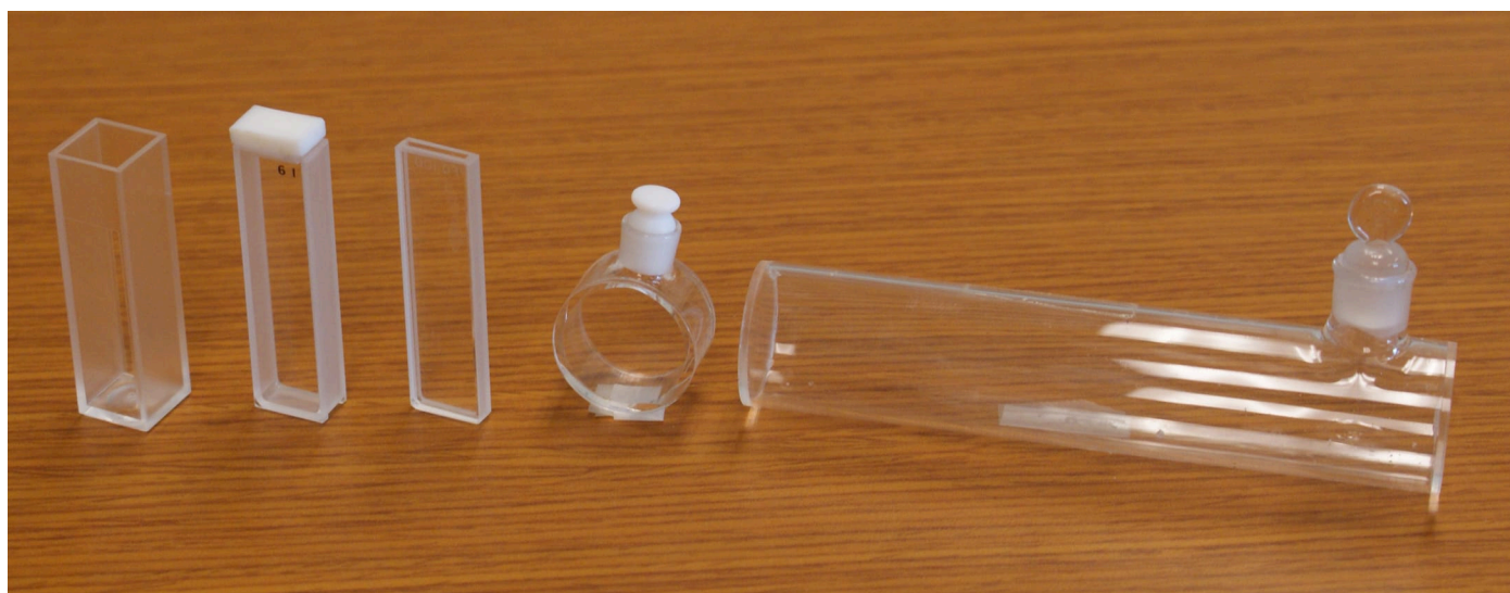
Figure 6.1.5.6 . Examples of sample cells for UV/Vis spectroscopy. From left to right (with path lengths in parentheses): rectangular plastic cuvette (10.0 mm), rectangular quartz cuvette (5.000 mm), rectangular quartz cuvette (1.000 mm), cylindrical quartz cuvette (10.00 mm), cylindrical glass cuvette with quartz windows (100.0 mm). Cells often are available as a matched pair, which is important when using a double-beam instrument.
