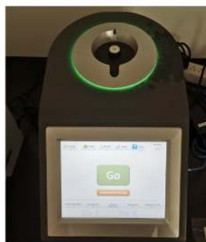
A model of bench top NMR: NMReady-60
