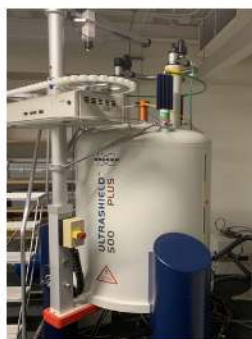
FT-NMR with superconducting magnet
