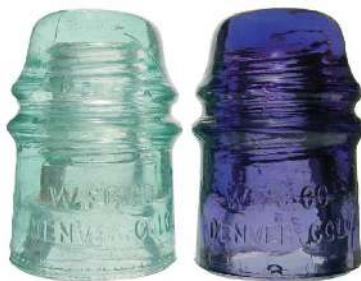
Figure 19.4.1: Radiation Damage. When high-energy particles emitted by radioactive decay interact with matter, they can break bonds or ionize molecules, resulting in changes in physical properties such as ductility or color. The glass electrical insulator on the left has not been exposed to radiation, but the insulator on the right has received intense radiation doses over a long period of time. Radiation damage changed the chemical structure of the glass, causing it to become bright blue. (CC BY-SA-NC; anonymous)
