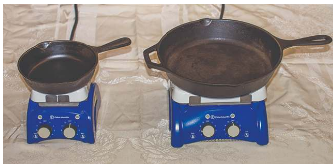
Figure 5.1.7: Due to its larger mass, a large frying pan has a larger heat capacity than a small frying pan. Because they are made of the same material, both frying pans have the same specific heat. (credit: Mark Blaser).
