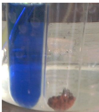
Figure 2: Fehling's test. Left side negative, right side positive. Image used with permission from Wikipedia
