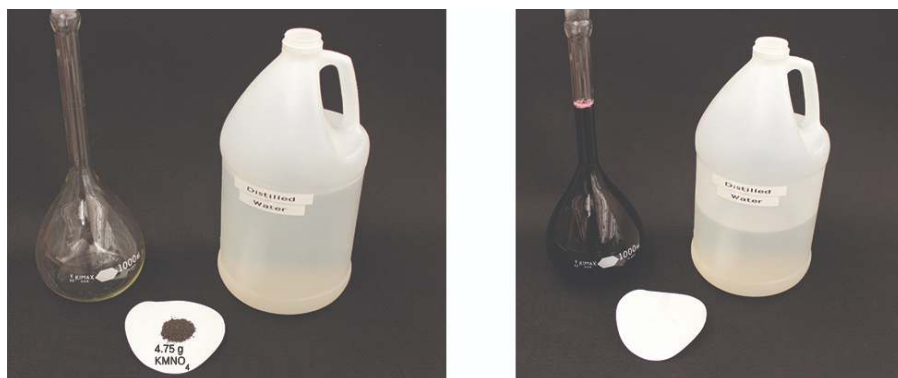
Figure 2.2.2.3: A solution of KMnO_4 is prepared by mixing water with 4.74 g of KMnO_4 in a flask. (credit: modification of work by Mark Ott)
