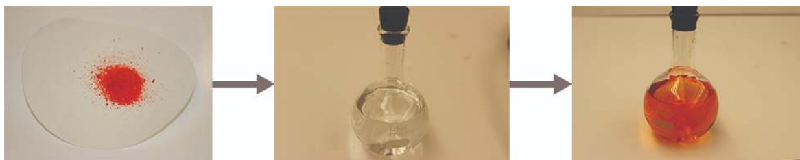
Figure 2.2.1.1: When potassium dichromate ( K_2Cr_2O_7 ) is mixed with water, it forms a homogeneous orange solution. (credit: modification of work by Mark Ott)
