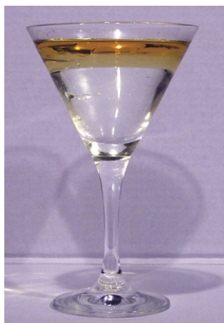
Figure 3.2.1.7: Water and oil are immiscible. Mixtures of these two substances will form two separate layers with the less dense oil floating on top of the water. (credit: "Yortw"/Flickr)
