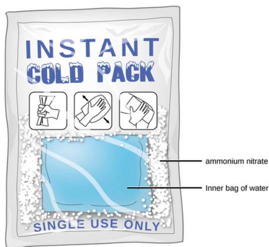
Figure 2.2.1.5: An instant cold pack gets cold when certain salts, such as ammonium nitrate, dissolve in water—an endothermic process.
