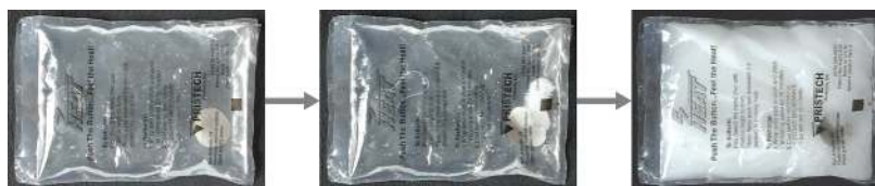
Figure 3.2.1.10: This hand warmer produces heat when the sodium acetate in a supersaturated solution precipitates. Precipitation of the solute is initiated by a mechanical shockwave generated when the flexible metal disk within the solution is “clicked.” (credit: modification of work by “Velela”/Wikimedia Commons)
