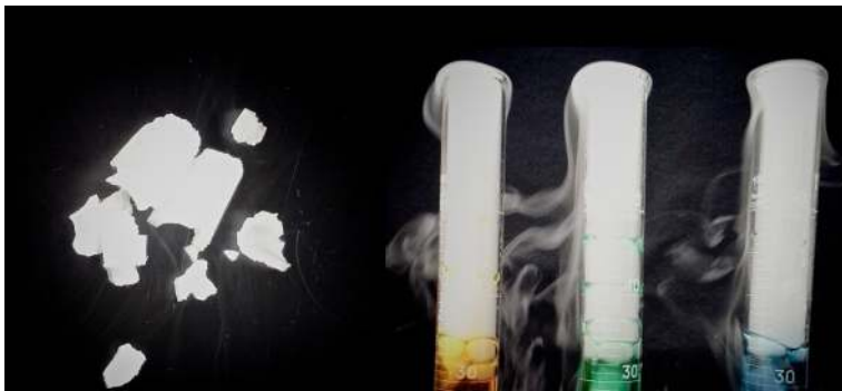
Figure 3.1.1.1: Solid carbon dioxide (“dry ice”, left) sublimates vigorously when placed in a liquid (right), cooling the liquid and generating a fog of condensed water vapor above the cylinder. (credit: modification of work by Paul Flowers)
