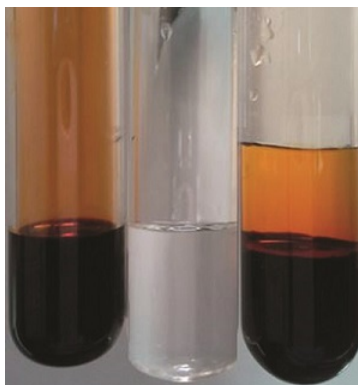
Figure 3.2.1.8: Bromine (the deep orange liquid on the left) and water (the clear liquid in the middle) are partially miscible. The top layer in the mixture on the right is a saturated solution of bromine in water; the bottom layer is a saturated solution of water in bromine. (credit: Paul Flowers)
