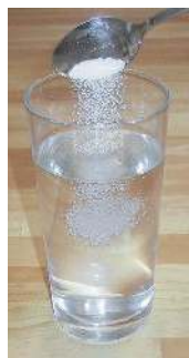
Figure 2.1.2.1 Making a saline water solution by dissolving table salt (NaCl) in water. The salt is the solute and the water the solvent. (CC-BY-SA 3.0; Chris 73).
