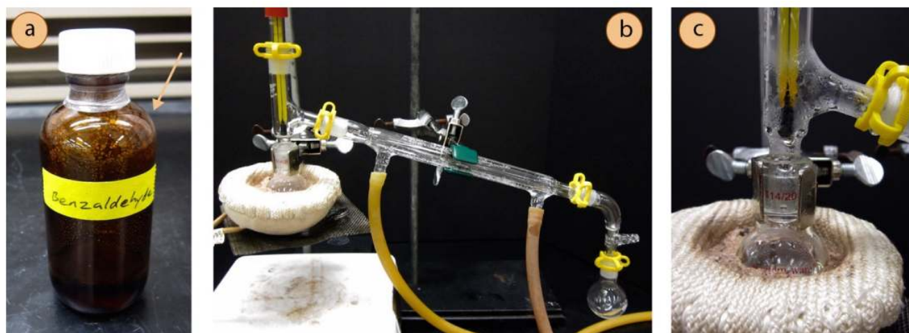
Figure 5.7: a) Benzaldehyde reagent with crystals of benzoic acid seen on the glassware (indicated with an arrow), b+c) Distillation.
