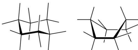
Figure 1.2.2.14 Chair (left) and boat (right) conformations for cyclohexane.
