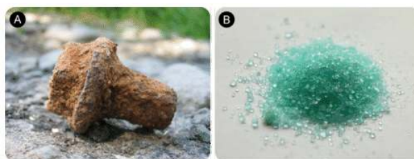
Figure 4.5.2: A. Rust is a complex combination of oxides of iron, among them iron (III) oxide, \text{Fe}_2\text{O}_3 . B. Iron (II) sulfate, \text{FeSO}_4 , has been known since ancient times as green vitriol and was used for centuries in the manufacture of inks. (CC by 2.0; Public Domain; (A) Paulnasca; (B) Ben Mills (Wikimedia: Benjah-bmm27) via (A) http://commons.wikimedia.org/wiki/File:Rust_screw.jpg ; (B) http://commons.wikimedia.org/wiki/File:Iron%2528II%2529-sulfate-heptahydrate-sample.jpg )
