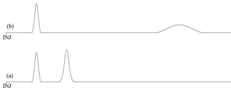
Figure 4. Elution of compounds where the \alpha -value in (b) is much greater than the \alpha -value in (a).
