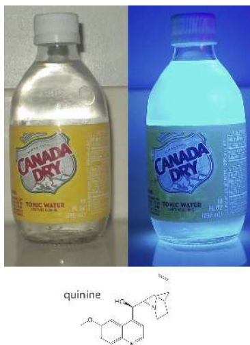
Figure 10.6.3 . Tonic water, which contains quinine, is fluorescent when placed under a UV lamp. Source: Splarka (commons.Wikipedia.org).
