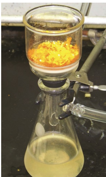
Figure 5.5.2: Precipitate may be removed from a reaction mixture by filtration.
