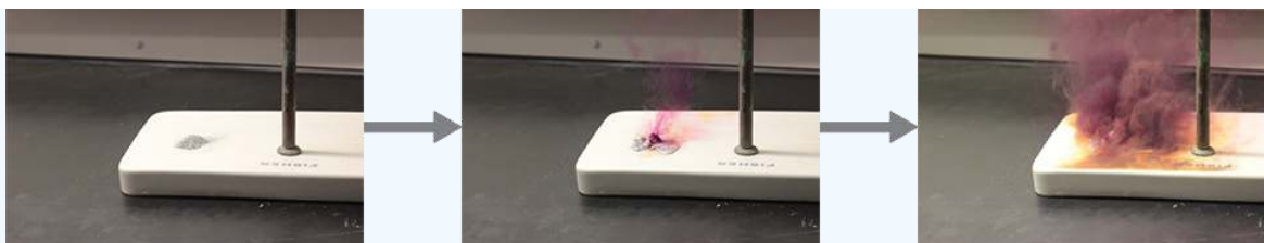
Figure 7.2.1: Aluminum and iodine react to produce aluminum iodide. The heat of the reaction vaporizes some of the solid iodine as a purple vapor. (credit: modification of work by Mark Ott)
