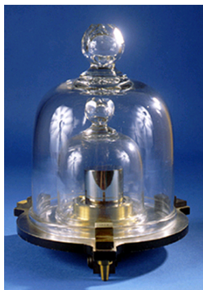
Figure 1.1.2: This replica prototype kilogram is housed at the National Institute of Standards and Technology (NIST) in Maryland. (credit: National Institutes of Standards and Technology).
