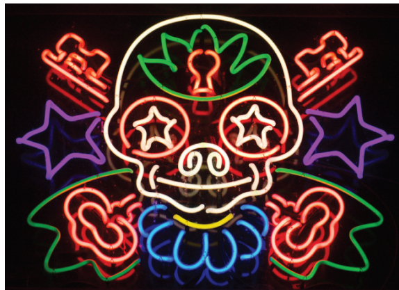
Figure 3.1.11: Neon signs operate by exciting a gas at low partial pressure using an electrical current. This sign shows the elaborate artistic effects that can be achieved. (credit: Dave Shaver)
