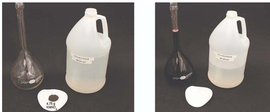
Figure 5.4.3: A solution of KMnO_4 is prepared by mixing water with 4.74 g of KMnO_4 in a flask. (credit: modification of work by Mark Ott)
