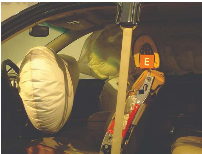
Figure 7.2.3: Airbags deploy upon impact to minimize serious injuries to passengers. (credit: Jon Seidman)
