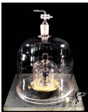
Figure 1: The Kilogram. The standard for the kilogram is a platinum-iridium cylinder kept in a special vault in France. Source: Photo reproduced by permission of the Bureau International des Poids et Mesures, who retain full internationally protected copyright.
