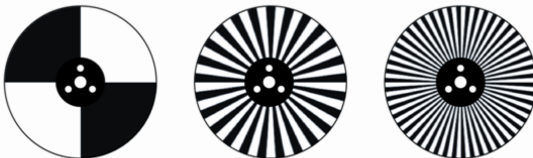
Figure 6.3B.11. Illustration of several chopper designs.
