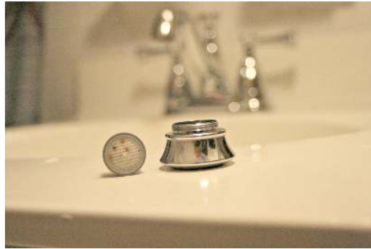
Figure 4.11: Faucet aerator illustration.
