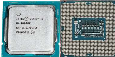
Figure 2.2.2: Left to right: Processor side of an Intel Core i9-10900K microprocessor showing the lid and markings for the processor. Image by Locke Cole is licensed under CC BY-SA 4.0 ; The back of the Intel Core i9-9900K. Image by PantheraLeo1359531 is licensed under CC BY-SA 4.0
