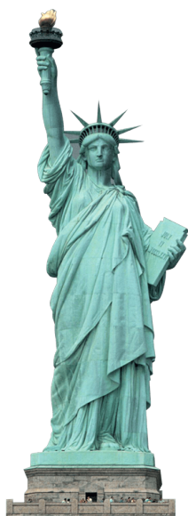
Figure 3.5.1: Green patina on the statue of liberty is a result of the oxidation of copper. Source: https://www.hiclipart.com/free-trans...hybox/download
