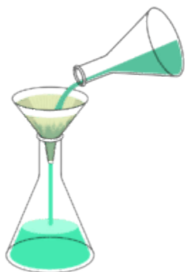
Figure 4.1.1: When a colored solution is passed through a filter, the entire solution, both solute and solvent, pass through unchanged.
