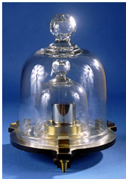
Figure 2.1.2: This replica prototype kilogram as previously defined is housed at the National Institute of Standards and Technology (NIST) in Maryland. (credit: National Institutes of Standards and Technology)
