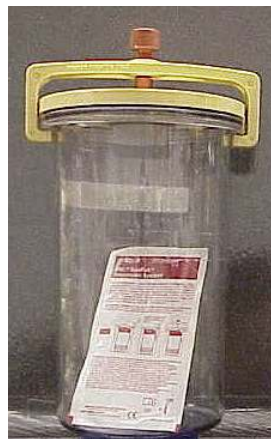
Figure 4: An anaerobic jar for cultivating obligate anaerobic species. Plates and test tubes with cultures to be cultivated in an anaerobic environment are added to the jar with a gas-generating pouch. The jar is then sealed. The gas generator pouch removes O_2 inside the jar. The jar environment then remains free of O_2 until the jar is opened.
