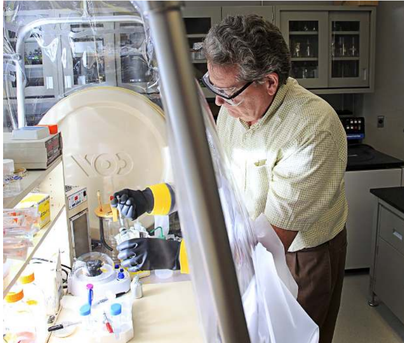
Figure 3: A microbiologist using an anaerobic chamber. Gloves reach into the chamber from outside of the chamber to conduct culture transfers and work with anaerobic bacteria. Inside of the anaerobic chamber there is a non- O_2 atmosphere and a catalyst system to remove any O_2 that might enter the chamber when samples and tools are transferred in and out of the chamber.
