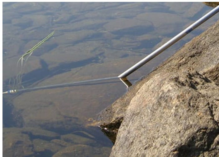
Figure 2.1.4: This straight pole appears to bend at an angle as it enters the water. This optical illusion is due to the large difference between the refractive indices of air and water.
