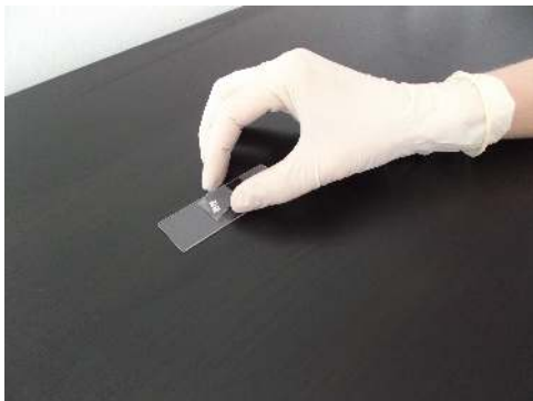
Figure 3. Making a wet mount. Note how the hand is placing the coverslip by dropping it at an angle. This helps prevent some air bubbles. Witia , CC BY 3.0 , via Wikimedia Commons
